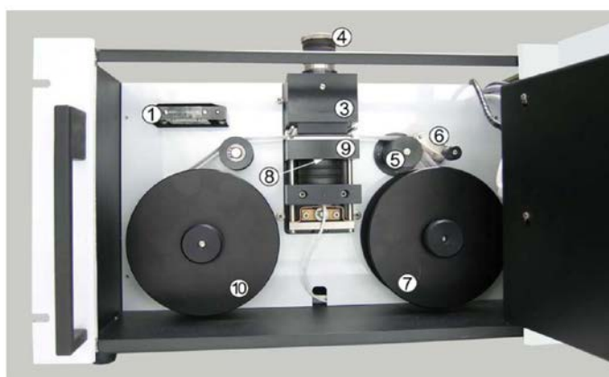
(1) reference gauge, (3) source holder, (4) fitting, (5) capstan, (6) disengageable pinch roller, (7) take-up reel, (8) Geiger-Müller tube detector, (9) pressure assembly, (10) pay-out reel.
