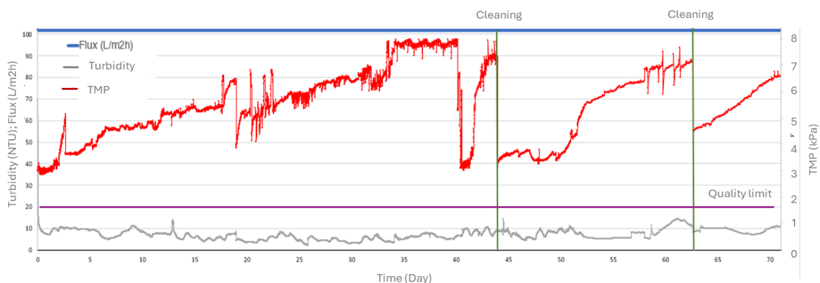
Figure 1. Evolution of TMP and turbidity profile during the filtration run.
