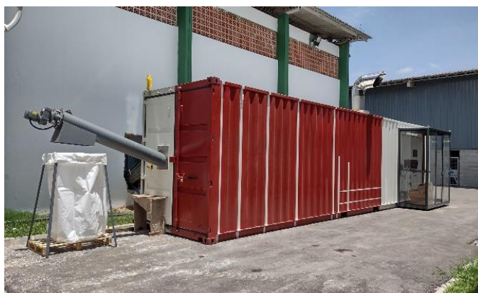
Figure 1: Small microwave dryer able to process WTP sludge
