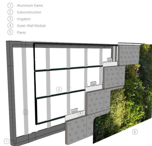
Figure 1: Scheme of Urbanscape® ornamental green wall tested irrigated with greywater (Source: Knauf Insulation Ltd.).
