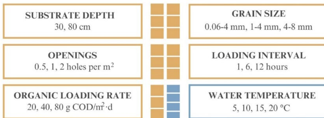
Figure 1. Operational and design parameters (in yellow), and water temperature (in blue) considered in the simulation study.
