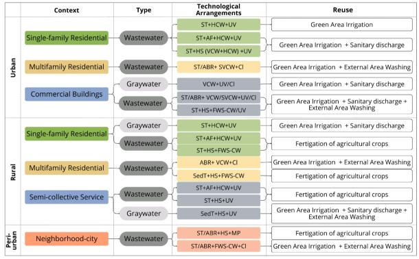
Note: ST: Septic Tank; HCW: Horizontal Flow Constructed Wetland; VCW: Vertical Flow Constructed Wetland; UV: Ultraviolet Radiation; AF: Anaerobic Filter; HS: Hybrid System (HCW+VCW); ABR: Anaerobic Baffled Reactor; SVCW: Saturated Vertical-flow Constructed Wetland; Cl: Chlorination; FWS-CW: Free Water Surface Constructed Wetland; SedT: Sedimentation Tank; MP: Maturation Pond.
